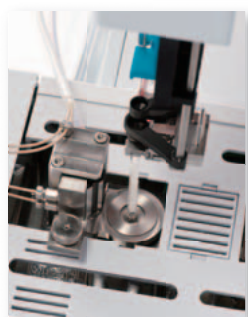
The liner is inserted.
